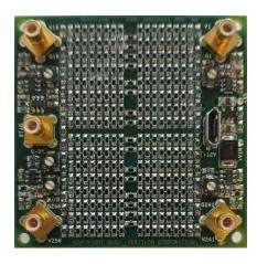
SIB71256 includes a high speed non-inverting preamplifier whose output is also available on an SMB connector. The polarity of the preamplifiers is such that the four anger and last dynode outputs produce all positive going signals.
