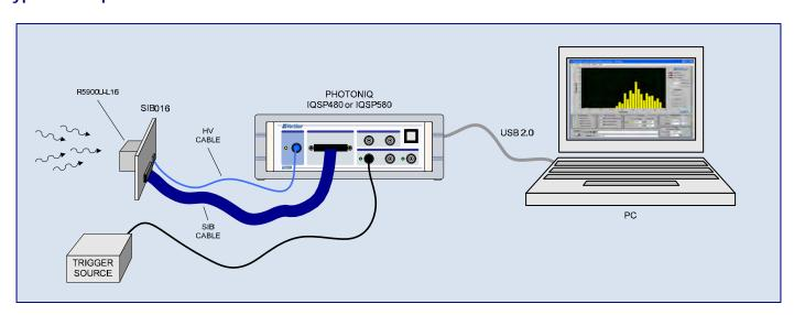
In a typical setup the Hamamatsu R5900U-L16 PMT is plugged into the SIB016 Sensor Interface Board which in turn connects to a Vertilon PhotoniQ IQSP480 or IQSP580 multichannel data acquisition system using a SIB cable. When triggered from an external source, the PhotoniQ integrates and digitizes the 16 charge signals from the R5900U-L16 and outputs a data packet to the PC over a USB connection. The PhotoniQ also supplies the PMT high voltage bias through a specialized high voltage cable.
