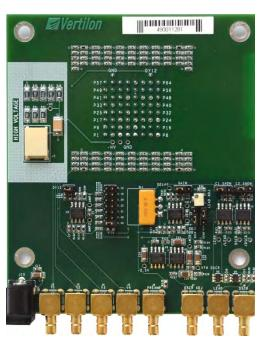
system or other external electronics. The outputs from a leading edge and zero slope discriminator — which respectively generate trigger signals based on threshold and pulse peak — are available on SMB connectors. Several user adjustments are included for optimizing system gain and trigger thresholds for the discriminators.
