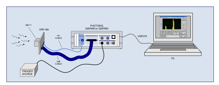
In a typical setup the Hamamatsu H8711 PMT is plugged into the SIB116A Sensor Interface Board which in turn connects to a Vertilon PhotoniQ IQSP480 or IQSP580 multichannel data acquisition system using a SIB cable. When triggered from an external source, the PhotoniQ integrates and digitizes the 16 charge signals from the H8711 and outputs a data packet to the PC over a USB connection. The PhotoniQ also supplies the PMT high voltage bias through a specialized high voltage cable.
