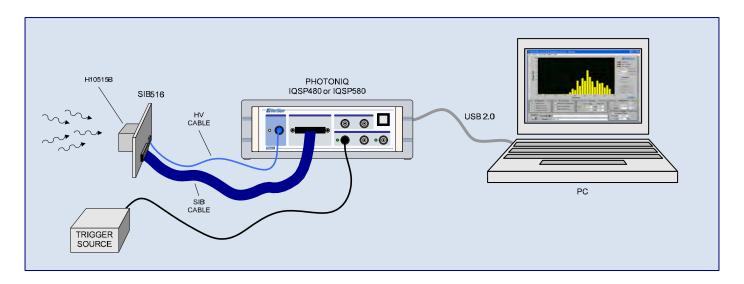
In a typical setup the Hamamatsu H10515B PMT is plugged into the SIB516 Sensor Interface Board which in turn connects to a Vertilon PhotoniQ IQSP480 or IQSP580 multichannel data acquisition system using a SIB cable. When triggered from an external source, the PhotoniQ integrates and digitizes the 16 charge signals from the H10515B and outputs a data packet to the PC over a USB connection. The PhotoniQ also supplies the PMT high voltage bias through a specialized high voltage cable.
