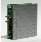
charge signal produced by the SiPM array. This signal is fed into a user-programmable leading edge discriminator that generates a trigger signal when an event exceeding a preset energy threshold is detected on the ArrayC-60035-64P device. The trigger output is typically connected to the trigger input on the PhotoniQ data acquisition system where it is used to initiate the collection of the energy signals from the SiPM array connected to the DAQ system's inputs.
