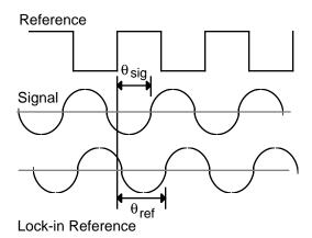
The SR830 amplifies the signal and then multiplies it by the lock-in reference using a phase-sensitive detector or multiplier. The output of the PSD is simply the product of two sine waves.
