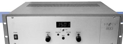
The PS-UVS20-A supplies all voltages and currents needed for the SPECS UVS 10/35 source operation. It consists of a switch mode power unit, an ignition unit and a fan control unit.
