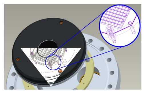
In the past delaylines were made of coils of thin wire wound around a base plate. Today, delaylines are based on a serpentine anode technology with improved high voltage decoupling. This technology leads, for example, to improved lateral resolution and linearity.
