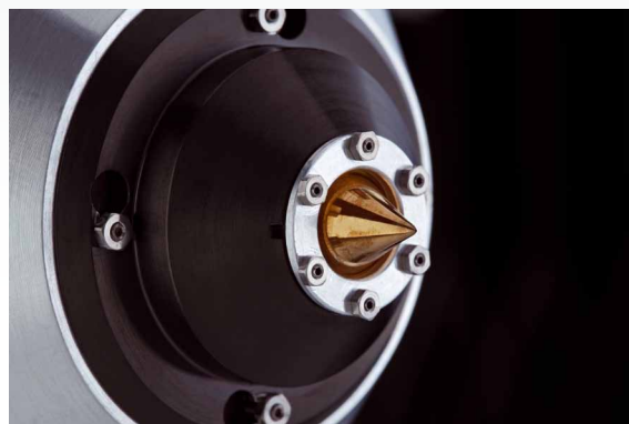
Exchangeable conic aperture separating the high pressure chamber from the first pumping stage. The diameter is 1 mm or less.
