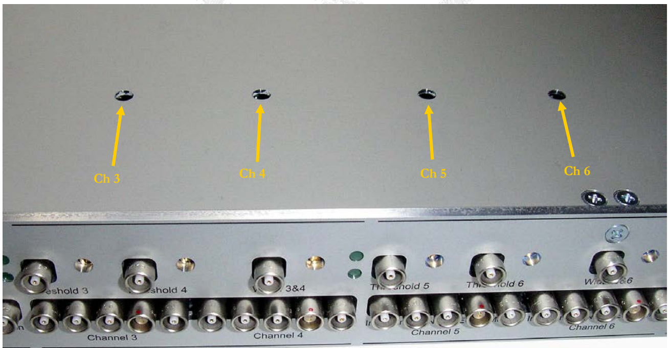
Figure 3.2: Top lid of ATR19 with holes to reach the gain potentiometers. Turning clockwise: amplifier gain is increased, turning counter clockwise: gain is decreased (for ATR19-2 refer to Chapter 3.6)
