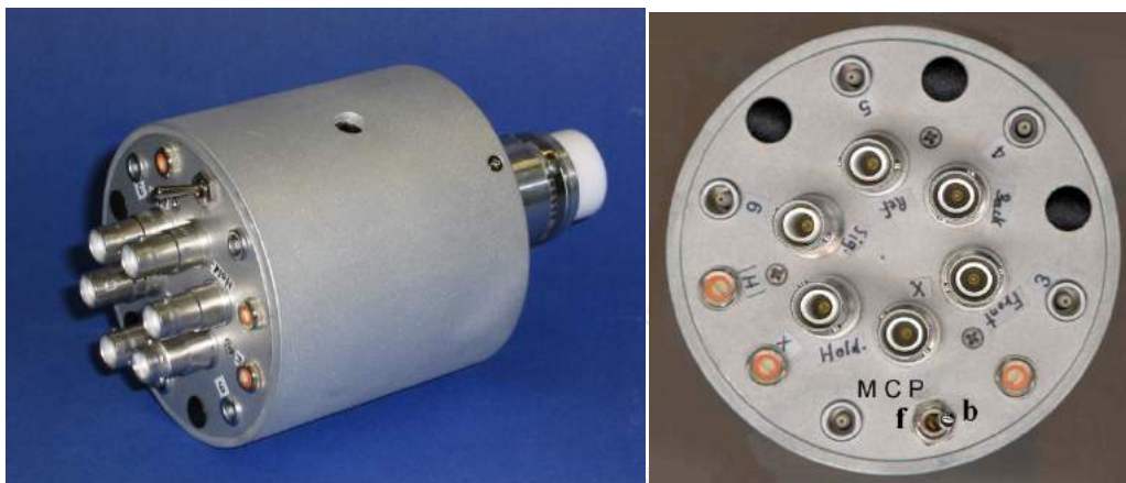
Figure 2.4: FT12TP Plug with switch for front (f) and back (b) MCP pickup. The hole in the ring case allows access to the in-line poti.
