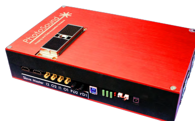
Example of ADC unit with 1x Cannon DLM260 AMP
