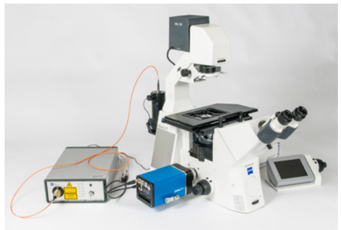
Figure 35: Microscope set-up example (Zeiss AxioObserver Z1, inverse widefield fluorescence microscope, courtesy of Zeiss AG) with Rapp OptoElectronic laser light source and combined de-speckling and optical coupling unit, with a pco.flim camera connected to the microscope and the laser light source.
