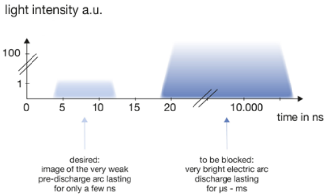
Figure 23: challenging light situation requiring highest extinction ratio.
