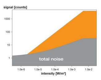
The upper curve (bright area) provides an example of the relationship between incoming light (x-axis: intensity), and the light signals that can be measured by a CCD camera (y-axis: signal). The lower curve (dark area) represents the total noise signal. The total noise signal is the sum of photon or shot noise, CCD noise and read out noise.
