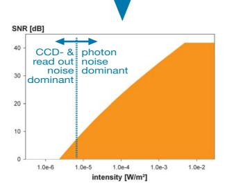
Using the two curves from the graph above, a corresponding snr-curve [dB] can be calculated, illustrated in the left graph. Although the numbers of the yaxis seem to be linear, it is clear from the unit [dB] that the scaling is logarithmic. The area below the curve indicates the maximum available dynamic range allowable for each amount of light that hits the CCD image sensor. The dotted line denotes the point where the photon noise is larger than CCD- and read out noise.
