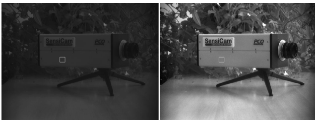
Figure 3 Left image: scaled to full scale 0 - 4095 => 0 - 255 Right image: scaled to minimum - maximum 167 - 1400 => 0 - 255 exposure time = 100 ms (for white rectangle see legend figure1)
