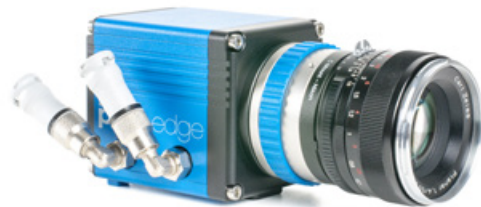
Water cooling unit Aquamatic II for use with pco.edge cameras.
