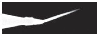
Fig. 1. «Whisker Type» probes specially designed for measurement of samples with near vertical sidewalls
