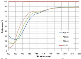
Reflectance of a mirror at three angles of incidence
