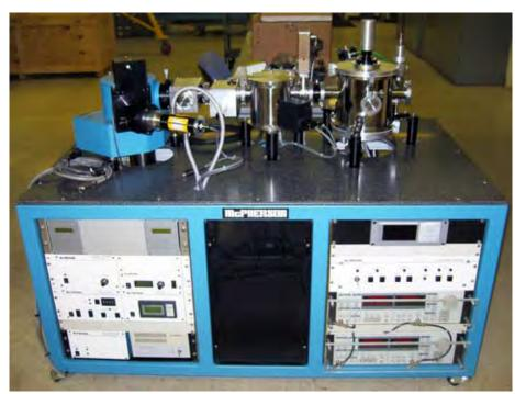
**VUVAS 2000 Vacuum Ultraviolet Analytical Spectrophotometer**
