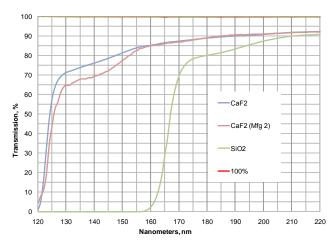
**Transmission** of crystalline Calcium Fluoride (from two different sources) and amorphous Fused Silica
