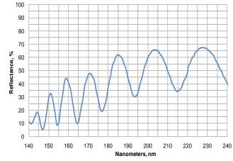
Thin film interference on a coated substrate
