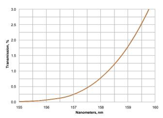
Transmission five scans at Fused Silica cut-on
