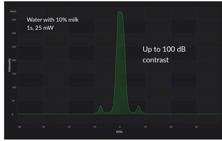
**Pump suppression** and **high contrast** (up to 100 dB): even highly turbid (opaque) samples can be measured
