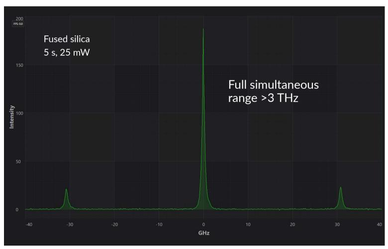
Large spectral range in a single snapshot (>1 THz): can measure hard materials and even ultra-low frequency Raman spectra
