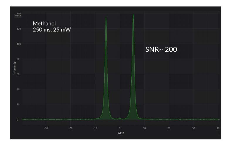
Fast and **effectively noiseless** Brillouin spectra with **minimal-to-no regular alignment** required
