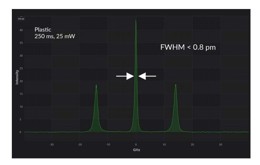
**High resolution**: <1 pm FWHM instrument response & <<0.05 pm precision on Brillouin shift measurement
