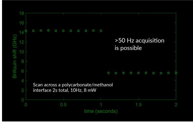
**Fast acquisition**: rapid scanning or monitoring of fast reactions (> 50Hz on demand)
