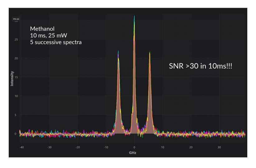
**Ultra-high throughput**: high signal-to-noise Brillouin signal in milliseconds is possible
