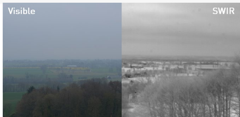
Visible versus SWIR imaging of a landscape in foggy conditions. Note how the view is much clearer and we can see some 10 km further in SWIR. Raw images acquired with a Nikon D5200 camera (left) and a C-RED 3 camera (right).
