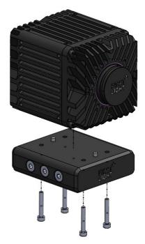
Schematic of hydraulic cooling plate installation
