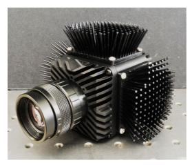
Passive heat sinks set-up
