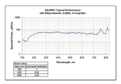
EQ-99FC Spectral Power with 230 µm Core Fiber Cable Assembly
