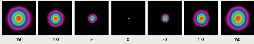
Fig 8. Typical beam profiles along propagation axis of FemtoLux 3 series laser
