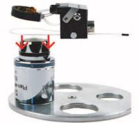
Place heater over objective then size for correct spacer
