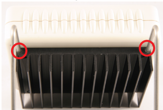
Locations to install controller stand
