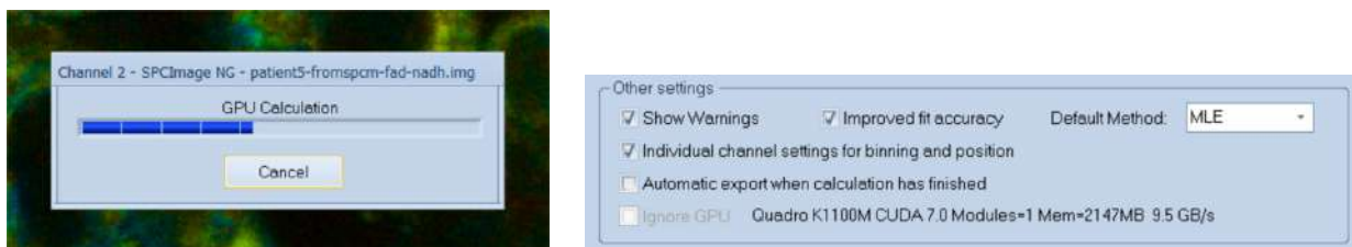
Fig. 7: Left: Progress panel during lifetime calculation, showing that GPU processing is used. Right: Part of 'Preferences' panel, indicating that a Quadro K1100M CUDA 7.0 device was found.
