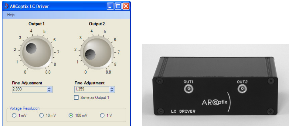
Figure 6: LC Driver with two independent outputs that are computer controlled via USB.
