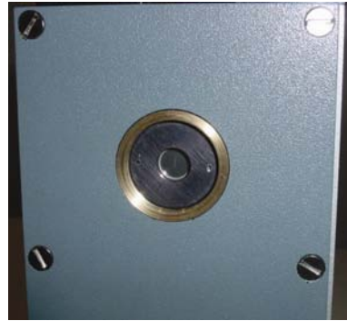
Figure 30: Shutter housing fitted with Slit Disc only
