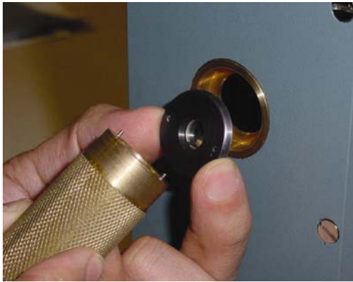
Figure 29: Inserting Slit Disc
