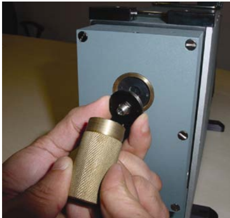
Figure 31: Fitting SMA connector over Slit Disc
