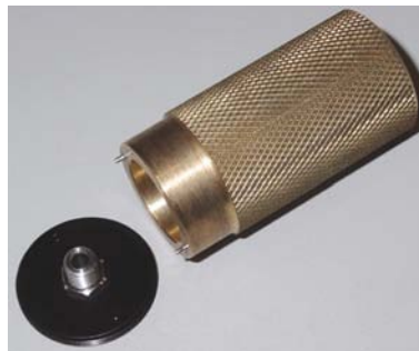
Figure 27: SMA connector & brass insertion tool
