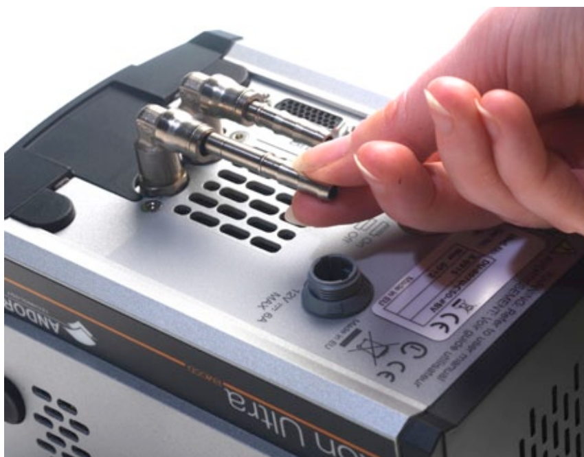
Figure 5: Removal of coolant hose inserts from quick release couplings on camera head
