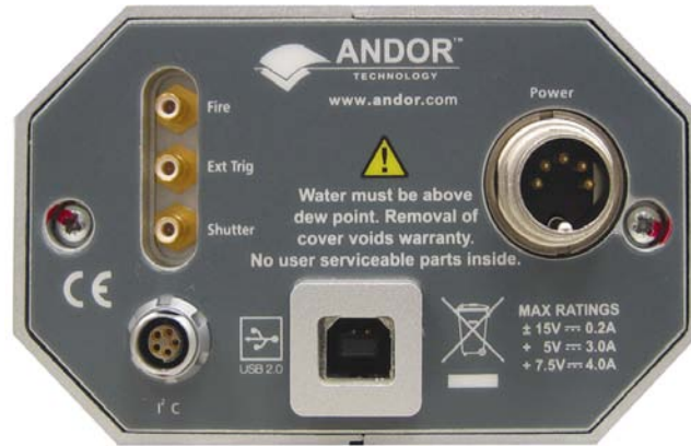
Figure 4: iDus backplate showing connections
