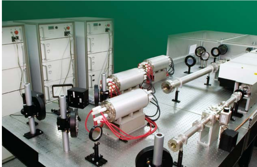
160 J @ 1053 nm MM laser system
