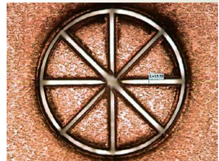
Copper removal from PCB with down to <math>< 20 \mu\text{m}</math> resolution.
