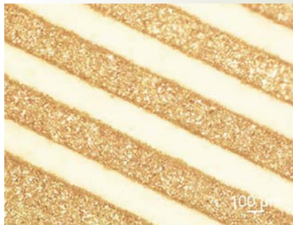
Ablation of 50 \mu\text{m} nickel layer from a ceramic substrate.
