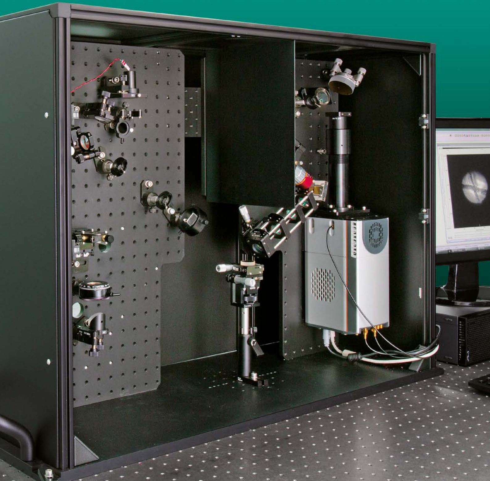
Photo: SFG microscope – provides spectral and spatial surface information with micrometers resolution
