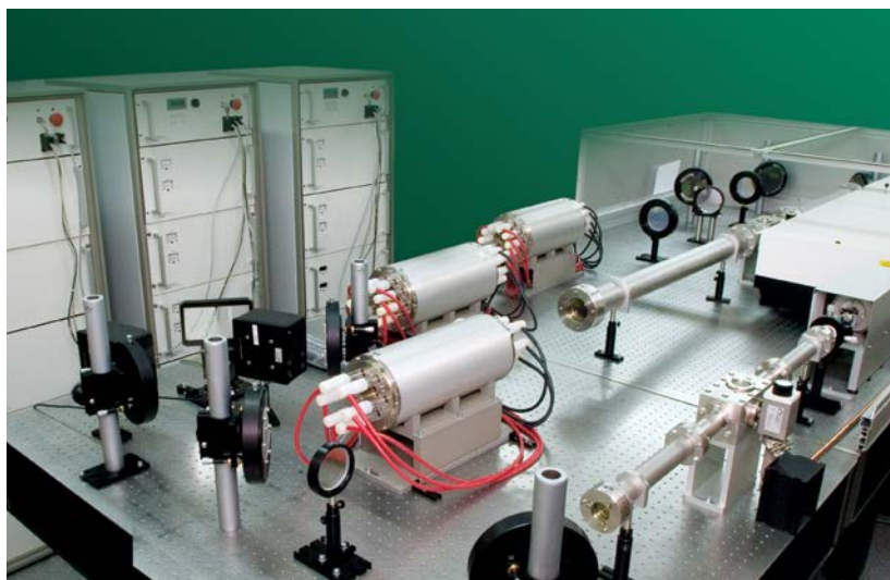
160 J @ 1053 nm MM laser system
