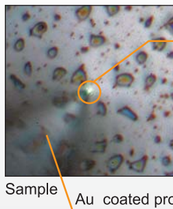
Microscopic image of the area around the AFM tip apex. Sample is visible even beneath the AFM probe because of very high NA of the microscope objective lens (0.7).
