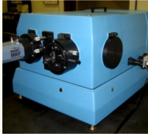
A 207 double pass - it doubles the 0.67-m focal length for dispersion and resolution equivalent to a 1.33m unit while maintaining f/4.7 aperture.
