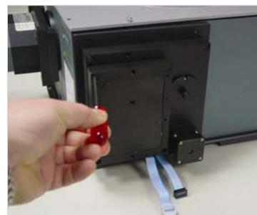
4. Connect the two ribbon cable connectors to the spectrograph PCB (note that the connectors are colour coded):
