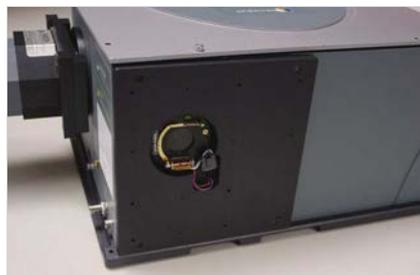
3. Attach the filter wheel housing noting the orientation relative to the spectrograph body then re-attach the motorised slit assembly to the filter wheel housing:
