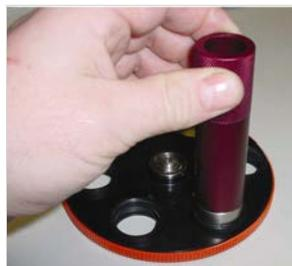
4. Remember to take a note of the filter details and the filter number where it has been fitted. These details will be required to update the filter details stored in the spectrographs non-volatile memory (see **page 20**). Re-attach the filter wheel in to the filter housing.
