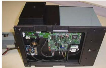
2. Remove the 25mm thick spacer block:
