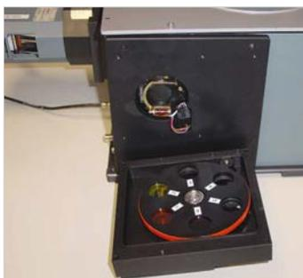
2. The filter wheel has been designed to allow the filter wheel to be removed from the filter wheel assembly housing with the removal of one screw. Unscrew the M5 x 16mm stainless steel Allen bolt from the middle of the filter wheel using a 3mm Allen key and withdraw the wheel from the housing:
