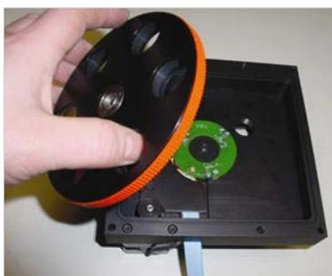
3. The filters may now be inserted into the filter wheel. Use the supplied filter ring wrench to first remove and then tighten the 1" filter retaining rings:
