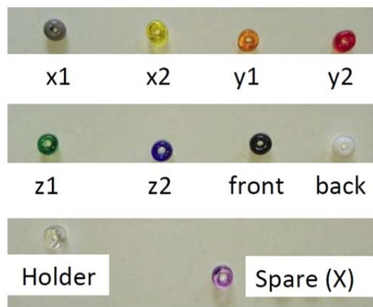
Figure 2.4: In-vacuum cable color code
