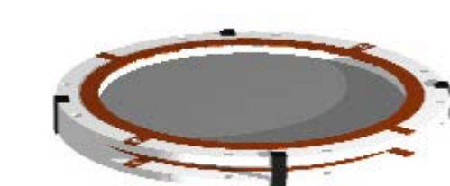
Figure 1.17: Assembly of MCP stack - Stage 3-4 (DLD40, DLD80 & HEX80)
