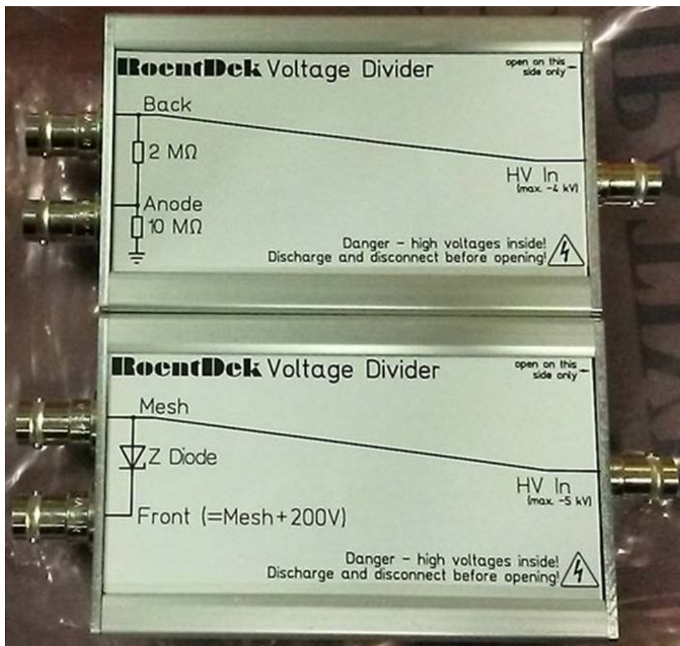
Figure 5.28: Set of voltage divider boxes for DET operated at high negative bias (MCP front up to -4800 V) with a mesh biased 200 V more negative than MCP front (lower box) and a resistor divider chain for biasing MCP back and Anode at adequate potential for single particle counting (upper box). The voltage drop between MCP back and Anode is 1/6 of the MCP back potential, here (can be altered by changing the 2 MΩ resistor, see Kirchhoff's laws).
