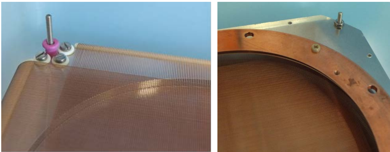
Figure 1.33: Special ceramic spacers (left picture) are placed on the rods protruding from the anode before the carrier plate is fixed to the anode holder with M2 nuts (right picture, here for DLD80).
