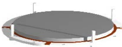
Figure 1.13: Assembly of MCP stack - Stage 2b (DLD40, DLD80 & HEX80/HEX75)
