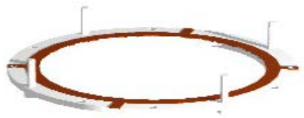
Figure 1.11: Assembly of MCP stack - Stage 1 (DLD40, DLD80 & HEX80)
