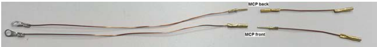
Figure 1.5: MCP connection cables for DLD with readily mounted option contain an intermediate connection coded male/female so that they can't be swapped (see above). It is important that the connection junctions don't get too close to each other ( > 3 mm distance) or to any other metal part after connections are in place and that they don't get close (see below). Extra insulation may be added.
