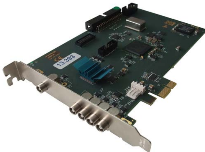
Figure 4.3: TDC4HM PCIe Card
