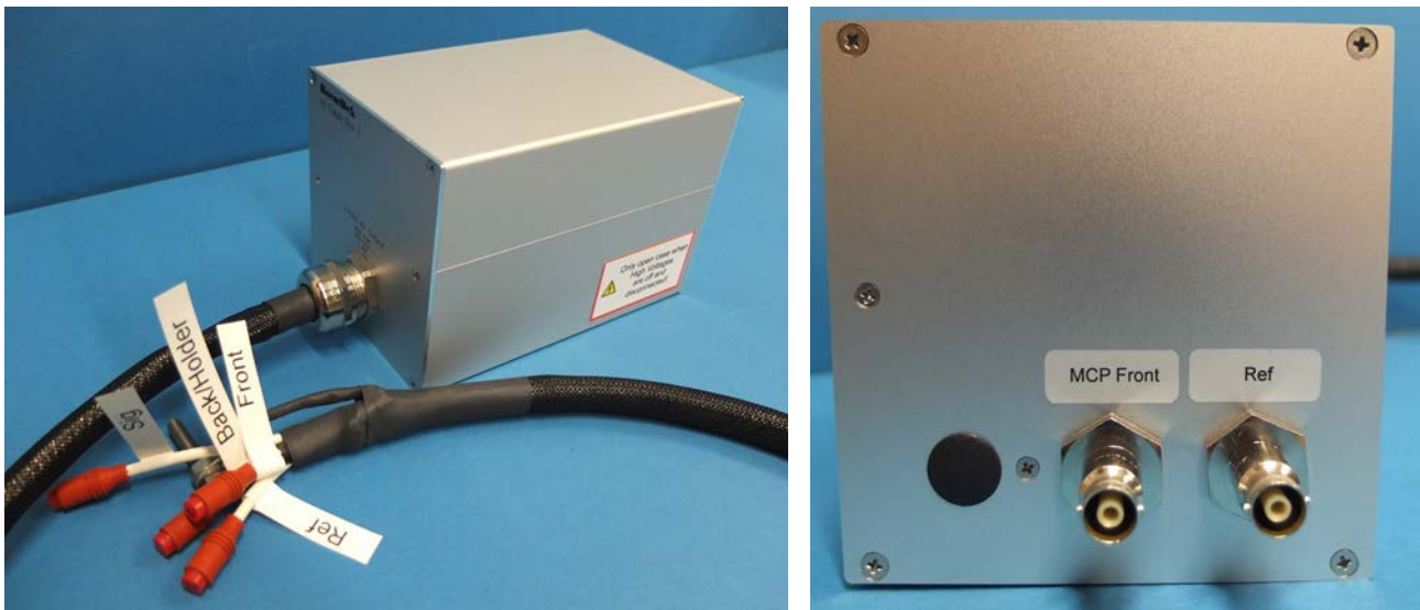
Figure 5.21: Left picture: HVZ10 box with four-fold high voltage output cable which will be connected to an XHV feedthrough. Right picture: high voltage inputs on rear panel. Here, two SHV10 socket are provided for supplying two independent voltages. Other versions are available which operate with just one input voltage (MCP front or U_{\text{ref}} ) and/or use other input socket standards
