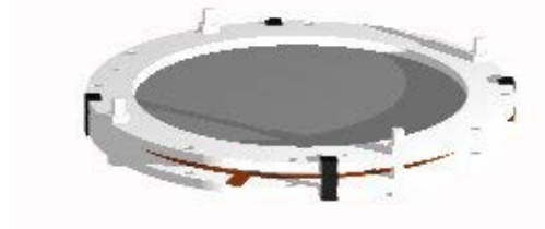
Figure 1.16: Assembly of MCP stack - Stage 3-3 (DLD40, DLD80 & HEX80)
