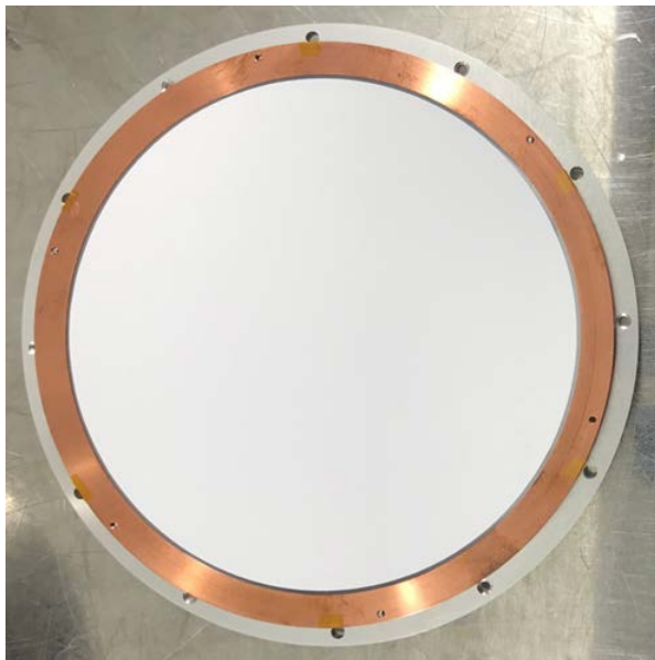
Figure 1.22: Left picture: the DET120P phosphor screen disc caged between metal rings, usually both of them electrically connected to the screen. Right picture: MCP back support plate with mounted screen and temporary centring ring for placing the MCP. The ring position is defined by the same guide pins as used during MCP mounting.
