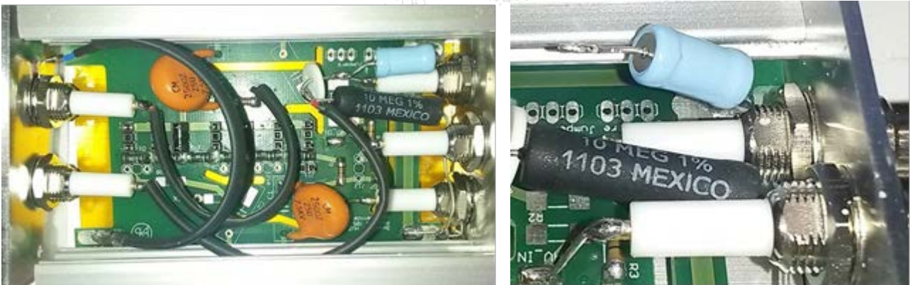
Figure B.4: HVZ-T4 versions with reconfigurable terminating resistance (pictures left above and below), or with fix 10 MΩ resistance (picture right above). If the unit is delivered with “T4” label (above) a 1 MΩ resistor is set parallel to the 10 MΩ resistor to ground (see picture left below). The total resistance is then 0.9 MΩ. By removing the solder connection as in picture right below the HVT resistance is changed to 10 MΩ. Additionally, a resistor bridge may be placed between Front and Back output sockets (backup resistor parallel to MCP stack).
