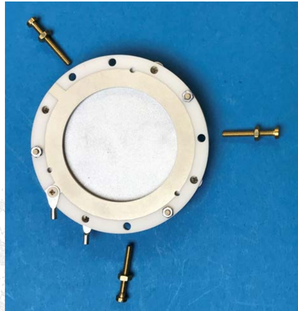
Figure 1.5: If the guide screws are placed in the front ring exactly as in the picture above (MCP contact side facing upwards) it is possible to place the anode/back ring without conflicts of occupied holes. Right: guide pin positions for alternative “bottom up” assembly.
