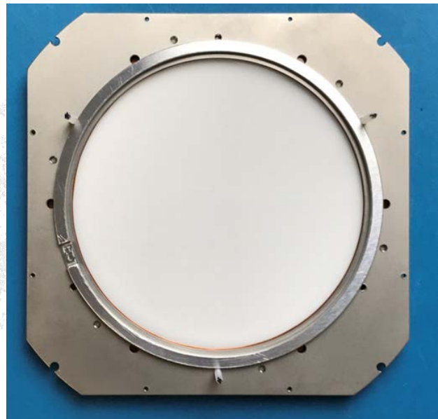
Figure 1.22: Left picture: the DET120P phosphor screen disc caged between metal rings, usually both of them electrically connected to the screen. Right picture: MCP back support plate with mounted screen and temporary centring ring for placing the MCP. The ring position is defined by the same guide pins as used during MCP mounting.
