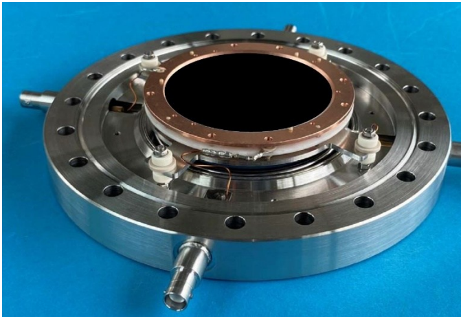
DET70P on “radial-type” window flange
