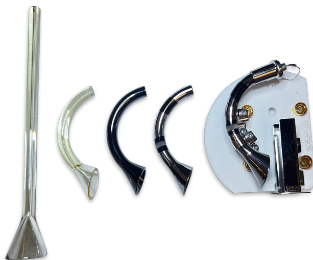
Fig. 2-3 CEM Fabrication Steps
