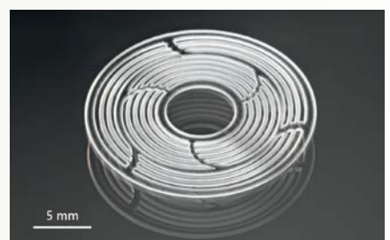
Thin fused-silica cutting. Courtesy of FTMC.
