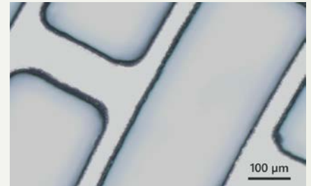
Kovar cutting. Courtesy of Laser Micromachining Ltd.
