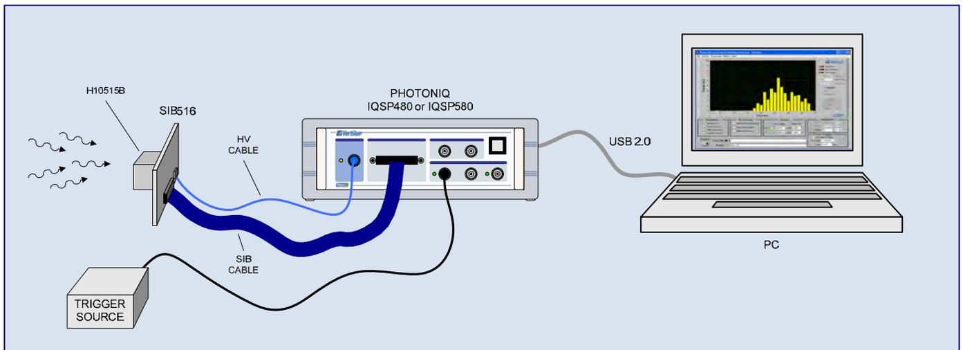
In a typical setup the Hamamatsu H10515B PMT is plugged into the SIB516 Sensor Interface Board which in turn connects to a Vertilon PhotoniQ IQSP480 or IQSP580 multichannel data acquisition system using a SIB cable. When triggered from an external source, the PhotoniQ integrates and digitizes the 16 charge signals from the H10515B and outputs a data packet to the PC over a USB connection. The PhotoniQ also supplies the PMT high voltage bias through a specialized high voltage cable.
