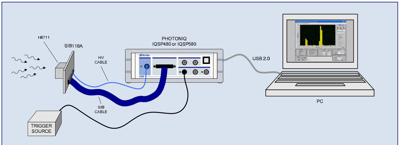
In a typical setup the Hamamatsu H8711 PMT is plugged into the SIB116A Sensor Interface Board which in turn connects to a Vertilon PhotoniQ IQSP480 or IQSP580 multichannel data acquisition system using a SIB cable. When triggered from an external source, the PhotoniQ integrates and digitizes the 16 charge signals from the H8711 and outputs a data packet to the PC over a USB connection. The PhotoniQ also supplies the PMT high voltage bias through a specialized high voltage cable.
