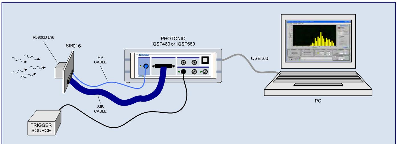
In a typical setup the Hamamatsu R5900U-L16 PMT is plugged into the SIB016 Sensor Interface Board which in turn connects to a Vertilon PhotoniQ IQSP480 or IQSP580 multichannel data acquisition system using a SIB cable. When triggered from an external source, the PhotoniQ integrates and digitizes the 16 charge signals from the R5900U-L16 and outputs a data packet to the PC over a USB connection. The PhotoniQ also supplies the PMT high voltage bias through a specialized high voltage cable.
