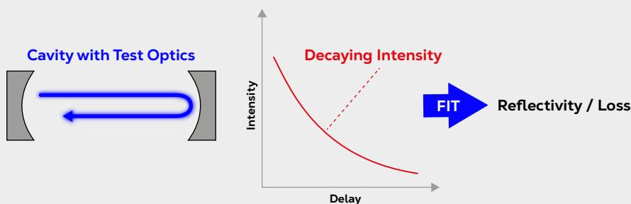
Sketch of the working principle of GLACIER, measurement and fitting procedure.
