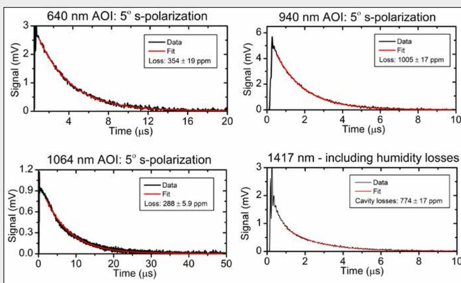
The figures show three typical measurements of high reflective samples and a measurement of an empty cavity (at 1417 nm) where humidity in the cavity causes extra losses. All measurements were recorded using the same GLACIER-C device, demonstrating its wavelength flexibility. The losses are obtained by measuring the cavity losses with and without the test sample. This provides an absolute measurement of the test sample.
