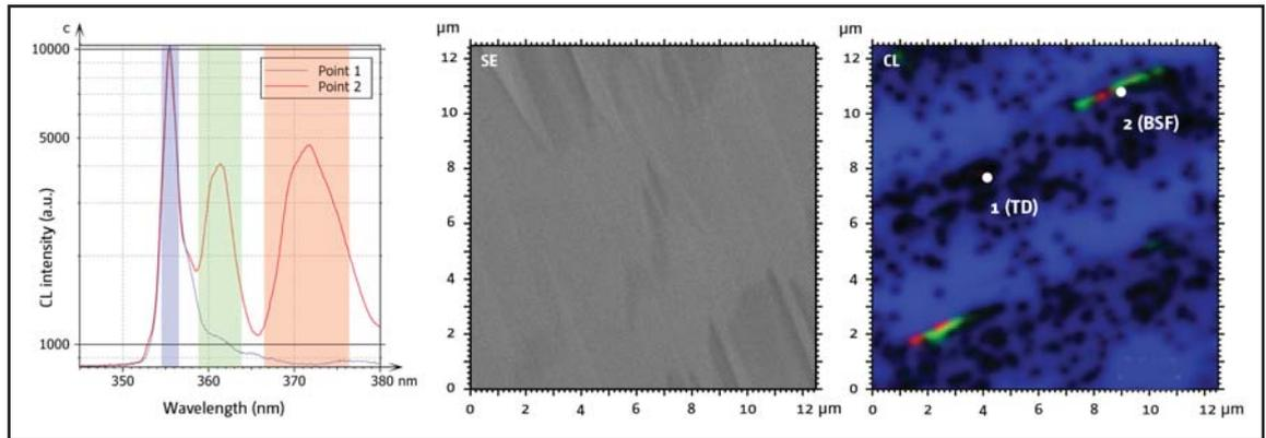
Note that a map can even be acquired by spacing out measurement points by hundreds of nanometres. So long as the spacing between measurement points is smaller than the diffusion length, the mapping technique will uncover defects. It is this feature that makes cathodoluminescence the ideal low-sampling technique for spotting loosely distributed defects without having to destroy the sample.
