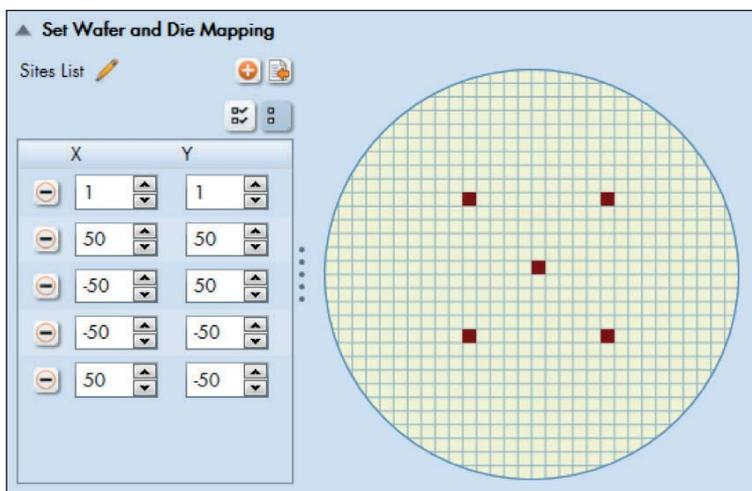
Figure 3. Wafer map showing a wafer with the user defined measurement locations.
