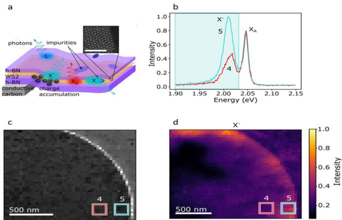
a) h-BN/WS<sub>2</sub>/h-BN heterostructure shows three emission lines: excitons (XA), trions (X<sup>-</sup>) and localized emitters (L). b) CL spectra for the regions highlighted in c and d. c) HAADF region measured in d and d) the X<sup>-</sup> intensity map revealing local trion enhancement.
