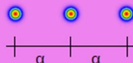
1x3 beam splitter diffracts the input beam into 3 beams. The power in each beam in ratio to the input power is > 28% and the uniformity error  $(I_{max} - I_{min})/(I_{max} + I_{min})$  is < 5%. The power in the highest unwanted diffraction order is < 3.5% (of input power).
