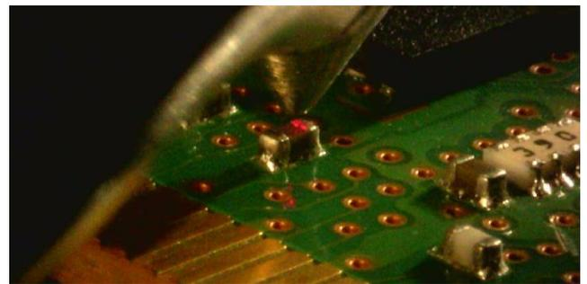
Fig. 6 Analysis position on the soldering joint
