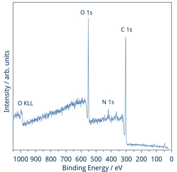
Fig. 10 Survey XPS spectrum of the coated PCB
