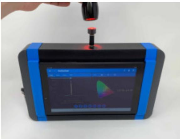
**LED Quality Control:** With so many LEDs being manufactured around the world you need a reliable instrument to test your incoming products. Checking the power and wavelength accuracy of specification and/or consistency is important!
