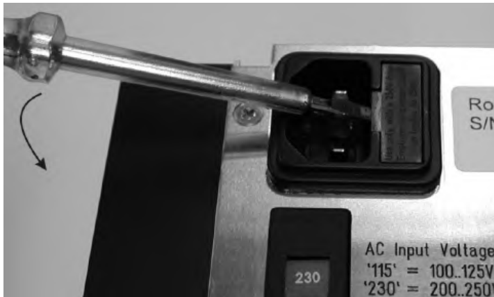
Figure 3.17: How to remove the input fuse
