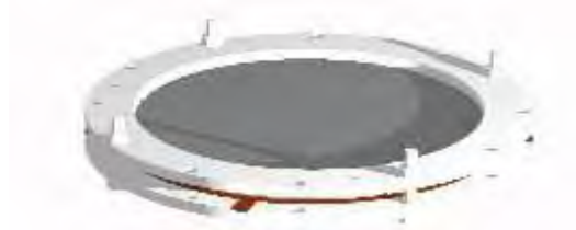
Figure 1.14: Assembly of MCP-stack - Stage 3-2 (DLD40, DLD80 & HEX80)
