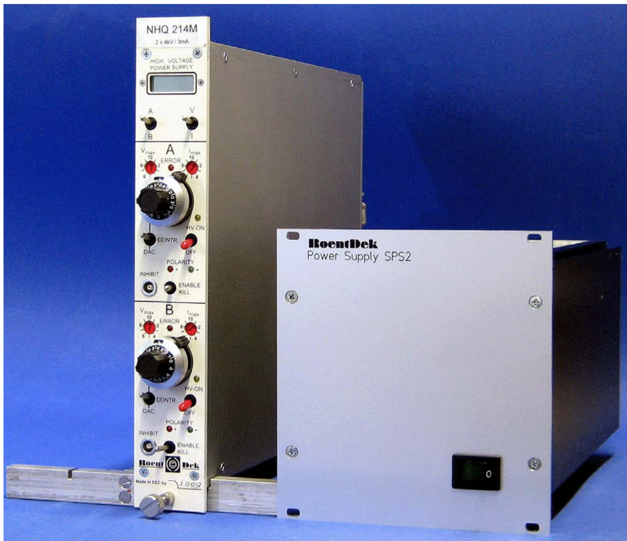
Figure 5.4: BIASET3 with SPS2 and one HV2/4 module (corresponds to BIASET3-2)
