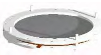
Figure 1.13: Assembly of MCP-stack - Stage 3-1 (DLD40, DLD80 & HEX80)
