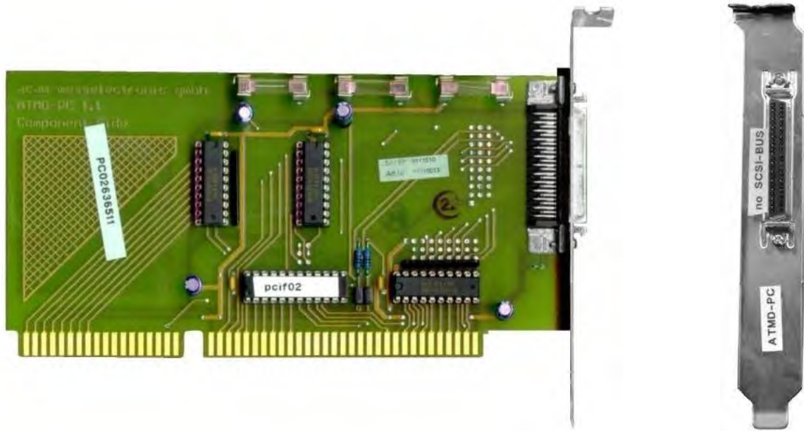
Figure 4.7: Side and input panel view of the HM1 - I/O-board (ISA)
