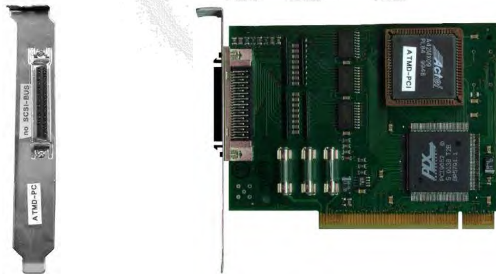
Figure 4.6: Side and input panel view of the HM1 - I/O-board (PCI)
