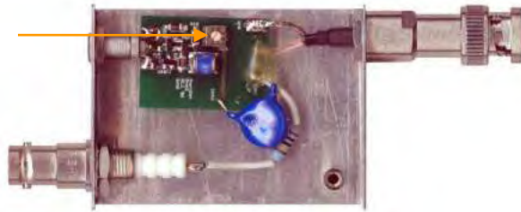
Figure 2.7: Single HF-signal-de-coupler plug (HFSD) with LEMO output and in-line poti
