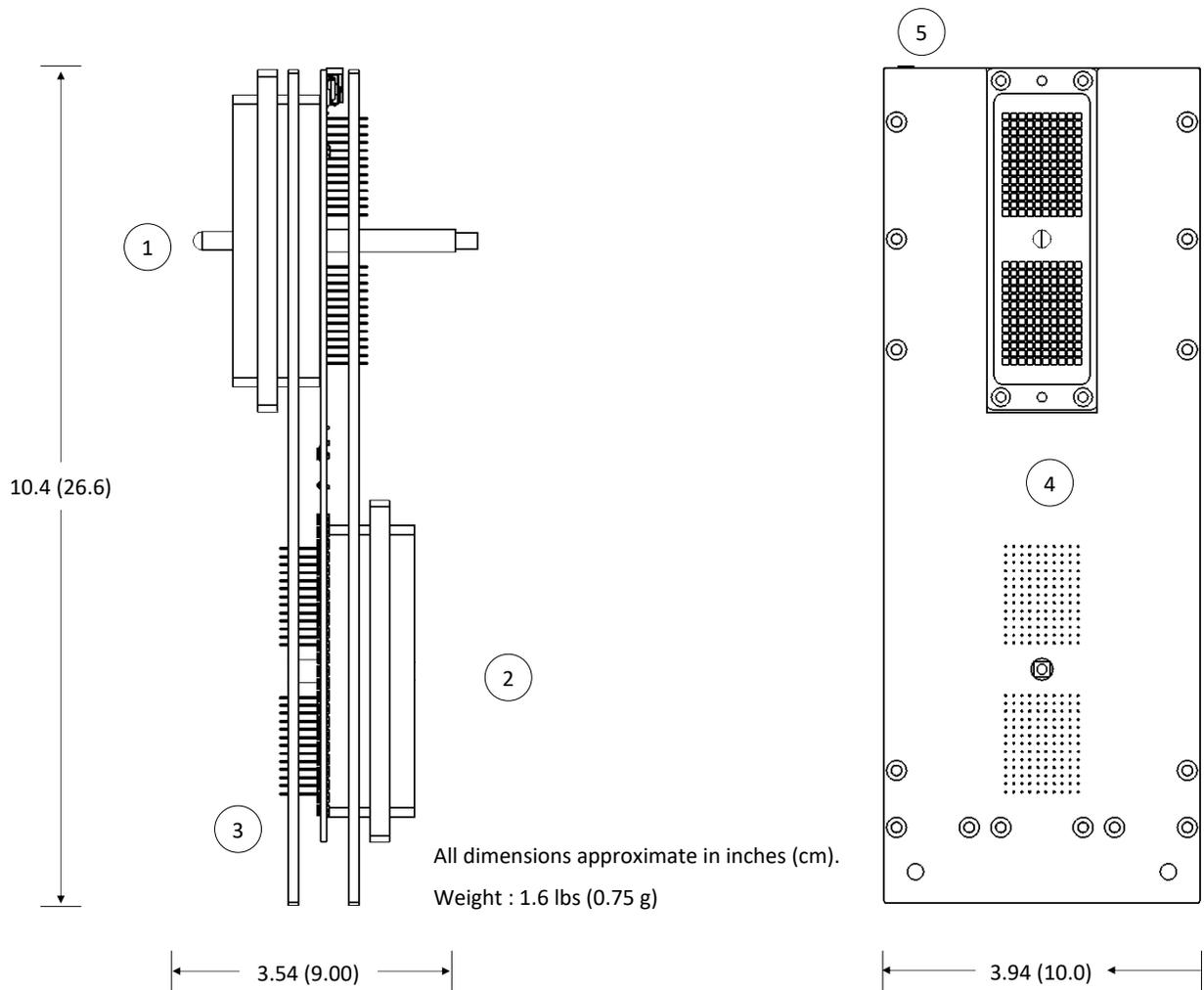
1. Medical grade Cannon DLM-260 probe input connector (pinout map available upon request). **Custom pin mapping to match existing third-party probes can replace default pinout map.**
