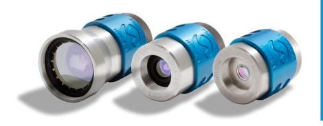
The HypIRia are wide-aperture, image-space telecentric lenses precisely crafted to provide clear and bright images in the SWIR spectral range. A broadband anti-reflective coating on carefully selected glass delivers high throughput and low-aberration imaging on an range extending from 1.0 to 2.9 µm.
